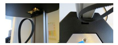
32. Finally, attach the belt to the bottom screw of the cart.
