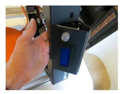
19. Position the bottom cover of your Tripodmaker Black Edition by holding the motor from the inside out. Insert the 6 screws to hold the bottom cover in place, but **don't tighten them yet**.
