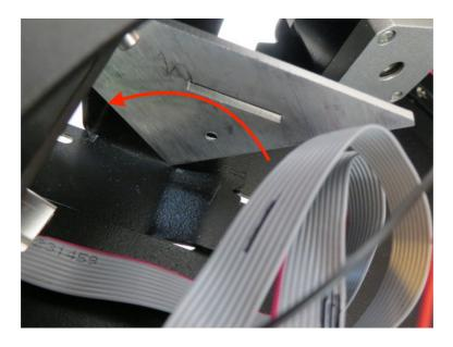
22. Reattach the LCD screen side panels with the big "+"-screwdriver.
