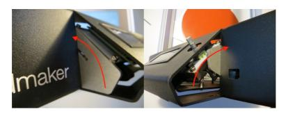
13. Unscrew the display from the frame by using the access holes on the bottom of your Tripodmaker Black Edition. You will have to squeeze your screwdriver next to the dismounted motherboard.
