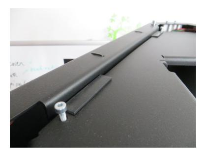
31. Connect the belt to the top screw of the cart and root the belt behind the returning pulley and motor pulley by using loops.
