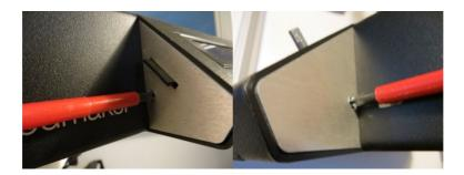
7. Remove the heated build platform by removing the countersunk 3 screws you find on the buildplate. It is advised to end with the top screw to prevent the plate from tipping during usncrewing.
