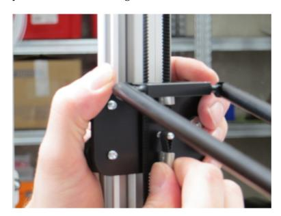
2. Remove the belts from your Tripodmaker Black Edition and remove the top cover of the printer
